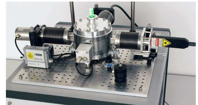
Advanced equipment for in situ monitoring of ultra-fast microwave heating processes
